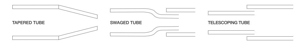
To calculate Telescoping Tube: Take the outer tube outside diameter (O.D.) measurement and subtract two times the wall thickness and the weld bead (0.5mm) to calculate the inside diameter (I.D.). i.e. 31.8 - (1.2 + 1.2) - 0.5 = 28.9, therefore tube 28.6mm O.D. will have 0.3mm clearance including the internal weld bead of the 31.8mm O.D. tube.
